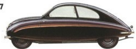
* The very first Saab – the 92001 – was a handmade prototype built in 1946, which, together with the second prototype – the 92002 – was shown to the press on June 10, 1947. It had a transverse twin-cylinder two-stroke engine, front-wheel drive, an aerodynamic design and a very rigid body.
